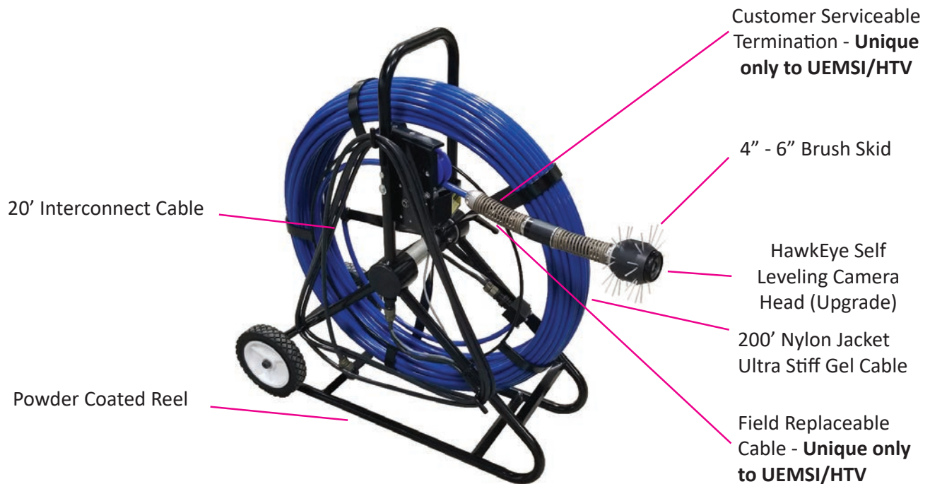
EagleVue Color Push Camera System shown with optional HawkEye self-leveling camera head, mechanical footage head and In-Line transmitter.
