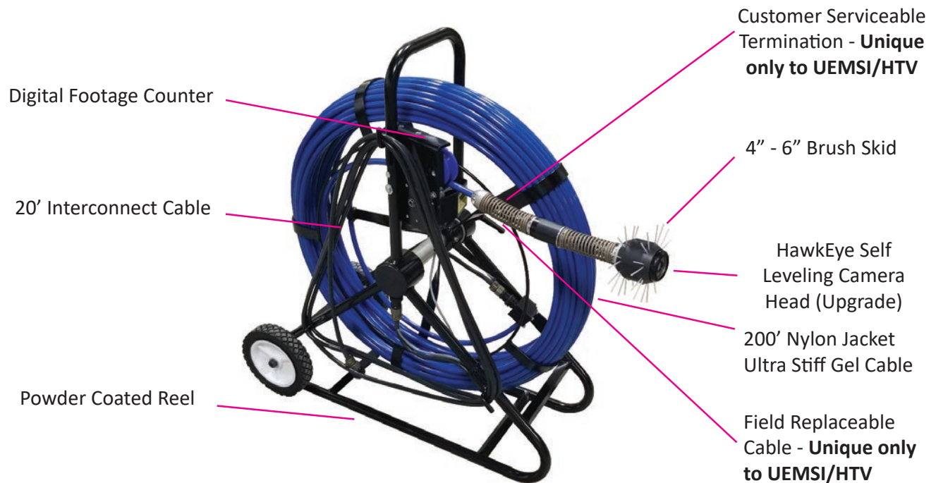
U-Vue Ultra Push Camera System, shown with optional HawkEye self-leveling camera head and optional In-line transmitter.
