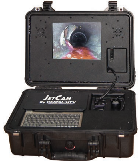
The Jet Cam PCU has a 10.4" sunlight readable color LCD monitor and can save data to a USB drive or SD card.
