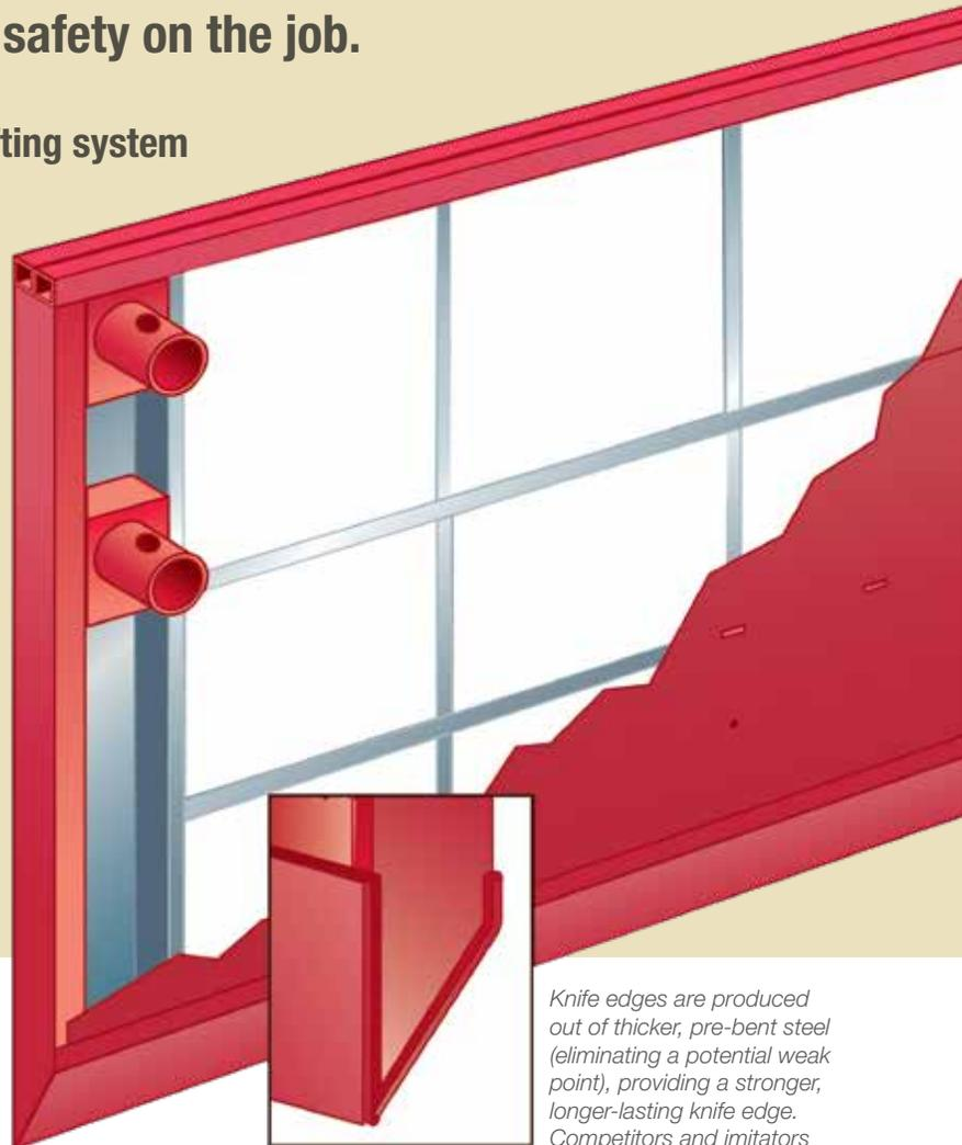
*Knife edges are produced out of thicker, pre-bent steel (eliminating a potential weak point), providing a stronger, longer-lasting knife edge. Competitors and imitators use an extension of the lighter gauge sidewall skin.*
