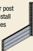
2. Set back panel, creating an "L". Install pins and keepers.
